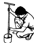
Figure 2. Place 10 to 15 soil cores into a plastic bucket; mix, dry, and transfer to a bag.
